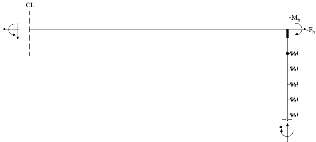
Figure 4-11: Idealization of Positive Temperature Gradient in SAP 2000 Models
