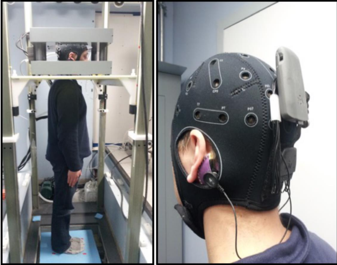
Figure 2-1 Stimulation apparatus. Volunteers stood in complete darkness, feet together, arms by their side and eye closed on a 1.5 cm foam pad covering the force plate. Their head was fully stimulated by Helmholtz-like coils centered on their ears, with ELF-MF stimulations at 8.89 T/s, 26.66 T/s and 39.98 T/s (left panel). The binaural bipolar DC montage stimulating both vestibular systems at 2 mA. The cathode is behind the right mastoid process and the anode is behind the left mastoid process (right panel).
