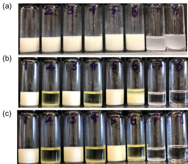
Figure 2.31 Photos of water-in-toluene emulsions. (a) After preparation (b) after 14 hours and (c) after 2 days. In photos, samples are arranged from experiment 1 to 8 ( Table 2.12 ) from left to right. The emulsions were destabilized upon the addition of glacial acetic acid, which triggered the depolymerization of the emulsifier, PEG-PEtG , while emulsions without glacial acetic acid remained stable and turbid over time.
