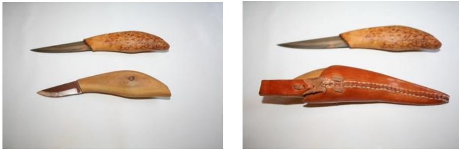
Figure 3 and 4: knives: birch (top), juniper (bottom). Leather sheath. Shaft molded to fit hand. The one on top tend to cut index finger when carving.
