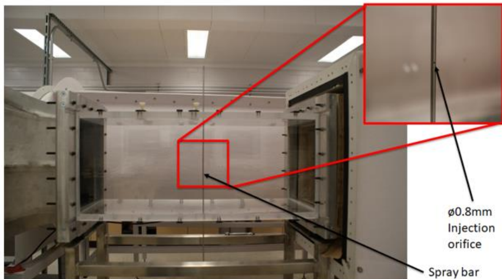
Figure 13: Setup of the spray bar in the test section
