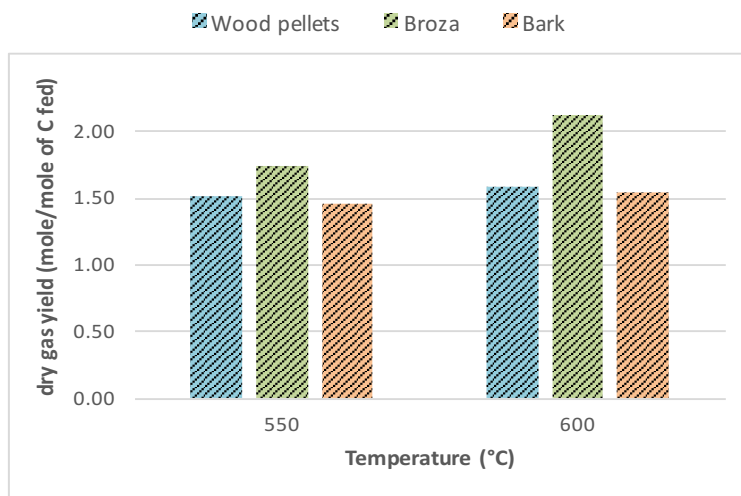
Figure 4.5. Changes of Dry Gas Yield with Temperature, from Steam-CO 2 Gasification of Wood Pellets, Bark and Broza. Gasifying agents: CO 2 at 1 atm and H 2 O at 0.5 atm. Data reported is the average of at least 15 repeats with a +/- 3-6% standard deviation.
