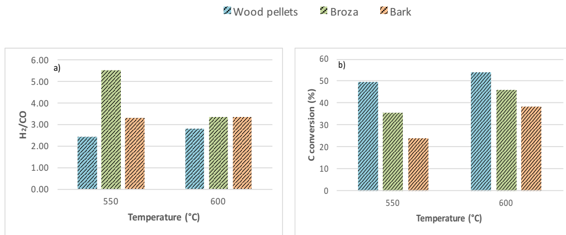
Figure 4.4. Changes of (a) H 2 /CO ratio and (b) the Conversion of Biomass Contained Carbon (CBCC) into synthesis gas with temperature during steam gasification of wood pellets, broza and bark under a He-water atmosphere. 40 min reaction time. Data reported is the average of at least 15 repeats with a +/- 3-6% standard deviation.
