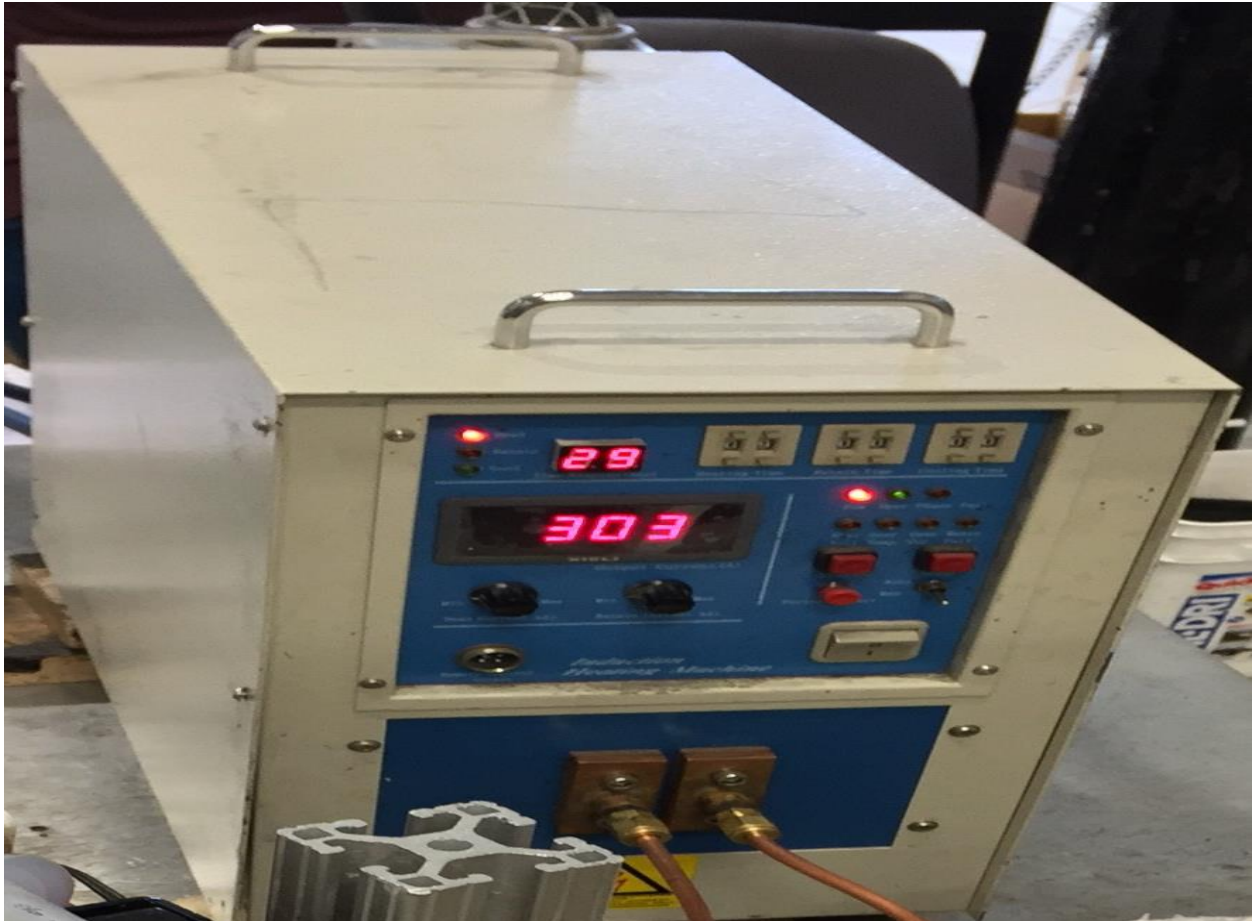
Figure B- 1.1: The Heat-Station of the induction heating system using IHM-2.
