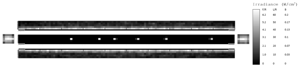
Figure 4.9 Detector data from the Zemax simulation of the row of concentrating features, showing light intensity patterns around the edges, and some illumination escaping the bottom face of the concentrator.
