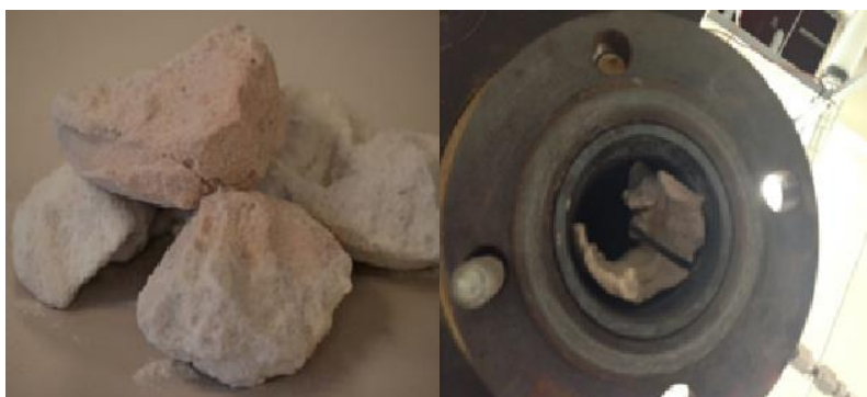
Figure 3-3 Formed agglomerates and the bottom view of the BFB reactor.
