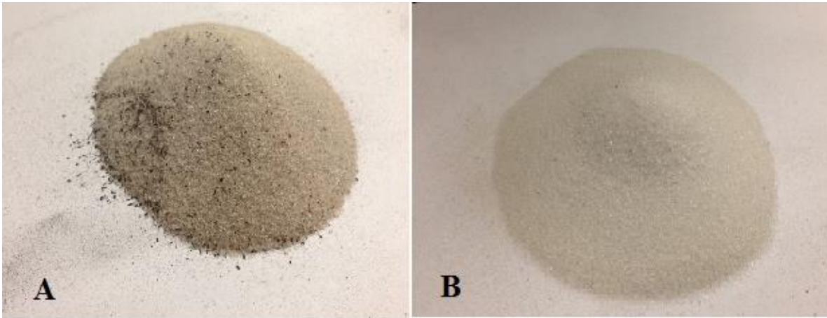
Figure 3-5 Photos of the bed material after the experiment with (A) and without (B) 0.6wt% KCl .
