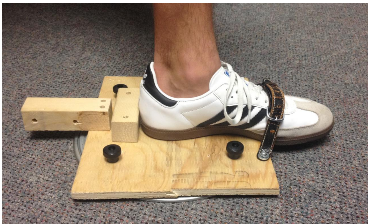
Figure 5: Rotating platform used for lead hip internal range of motion test
