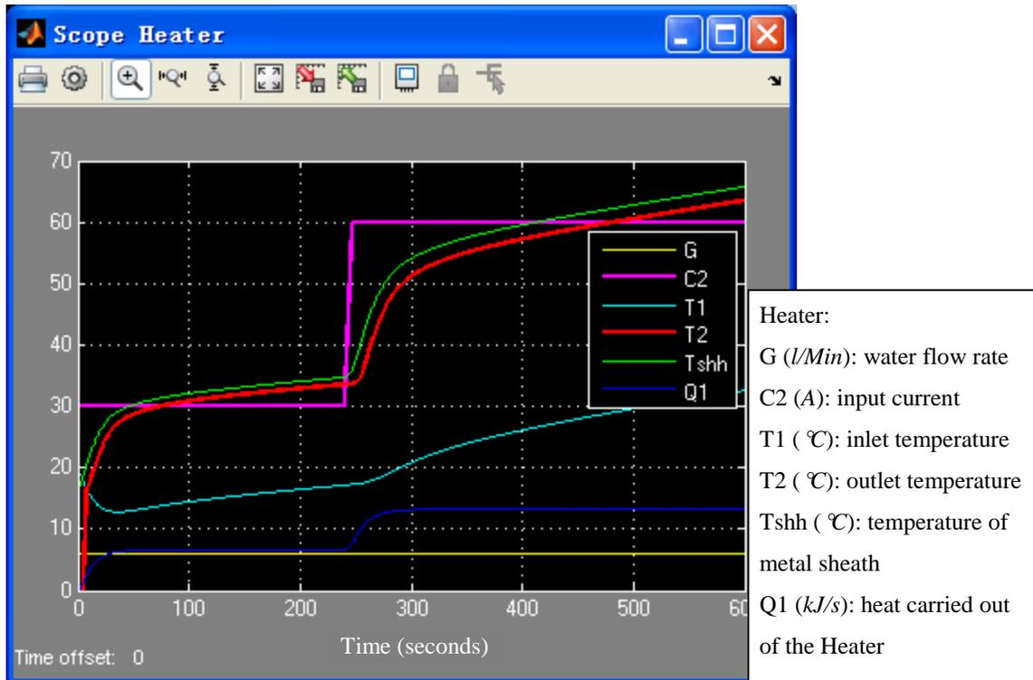
Figure 5-21 Monitoring of variables in the Heater
