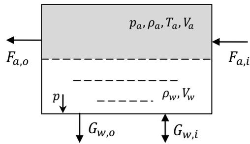
**Figure 2-9 Illustration of the Pressurizer model**
