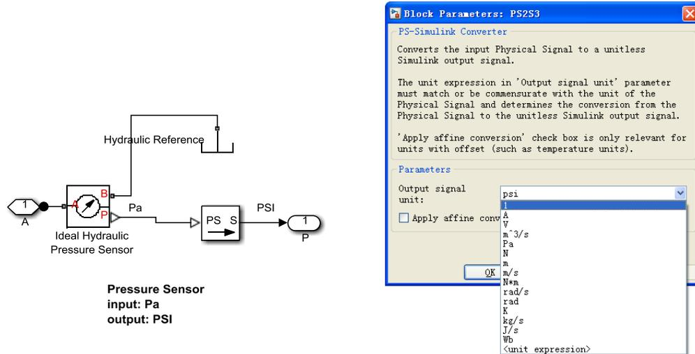
**Figure F-24 Output of hydraulic pressure sensor**
