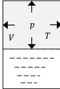
**Figure 2-4 Pressure of gas in a closed space**
