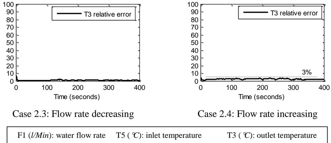
**Figure 5-8 Response of the flow rate varying to outlet temperature in the Chiller**
