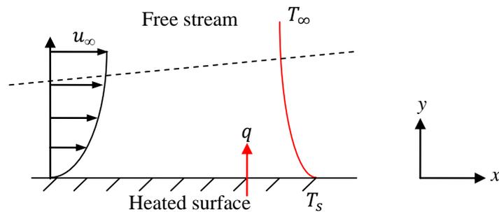
**Figure 2-5 Convection heat transfer**
