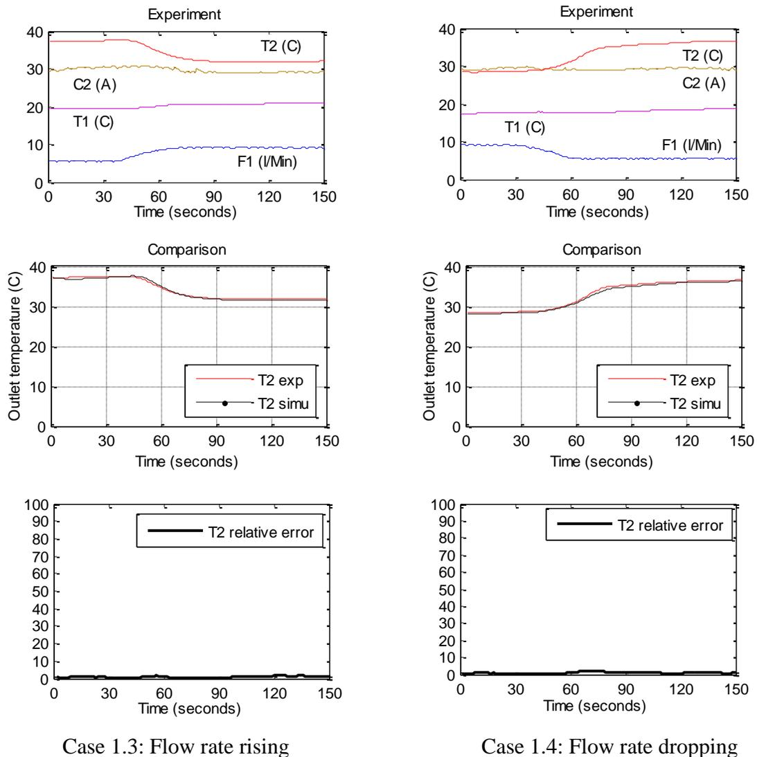
C2 (A): current F1 (l/Min): water flow rate T1 (°C): inlet temperature T2 (°C): outlet temperature
