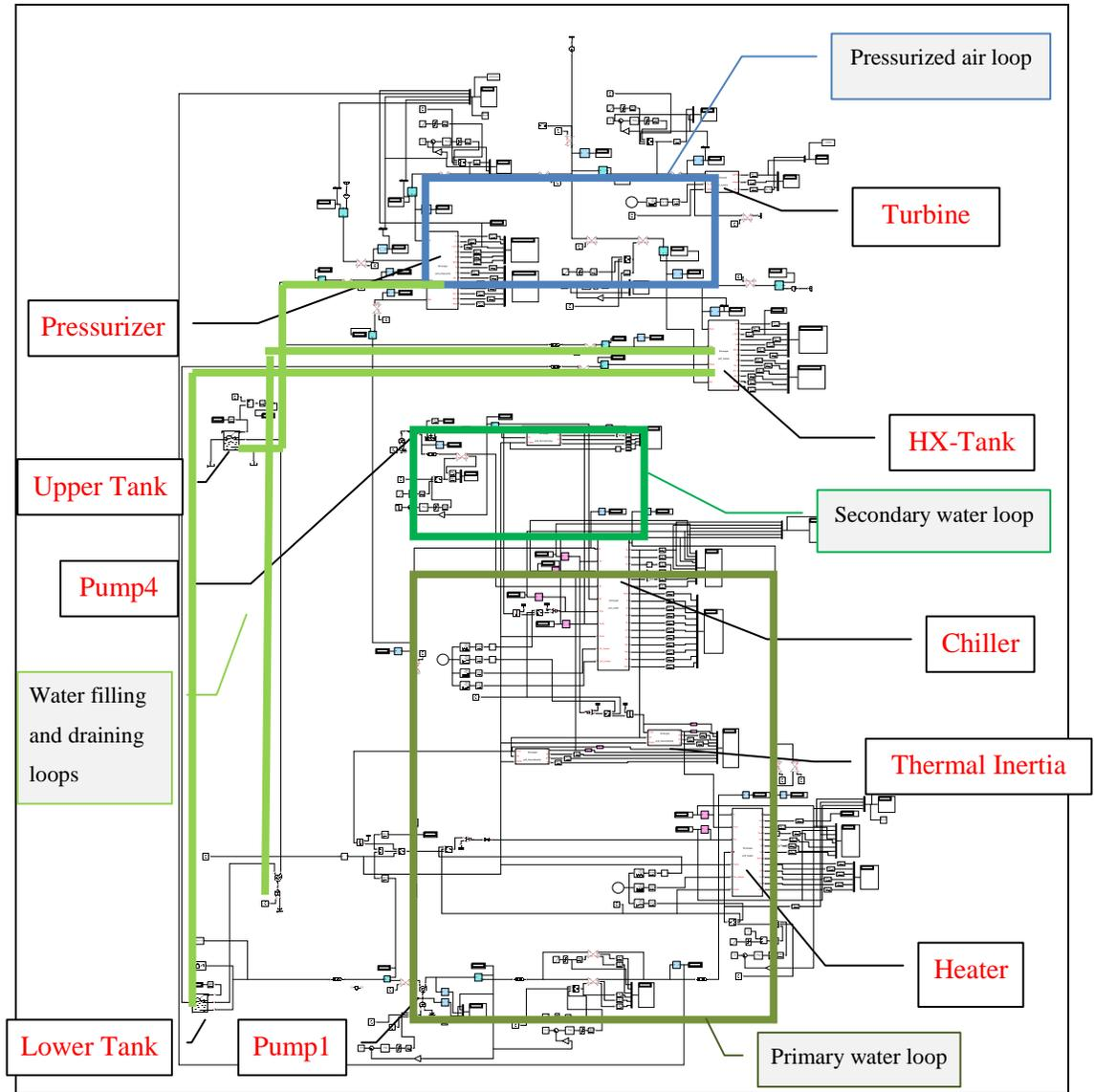
**Figure F-17 Overview of the simulator diagram**
