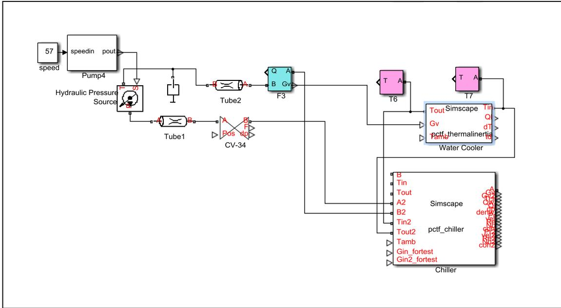
**Figure 4-4 Diagram of the secondary water loop**
