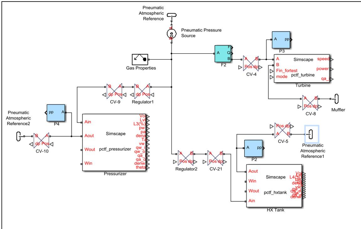
**Figure 4-5 Diagram of the pressurized air loop**
