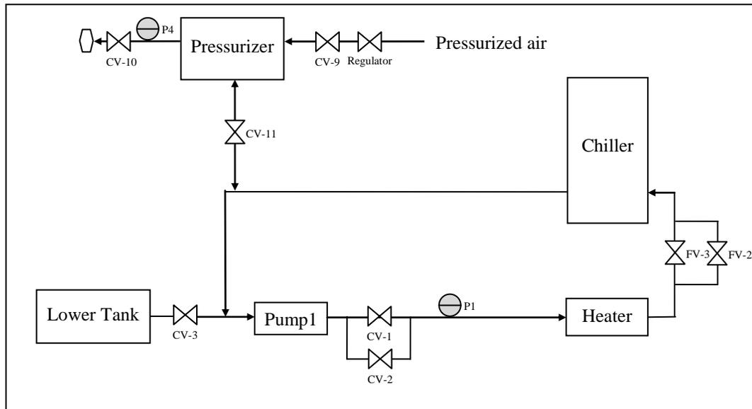
**Figure 5-19 Pressurizer and the primary coolant loop**
