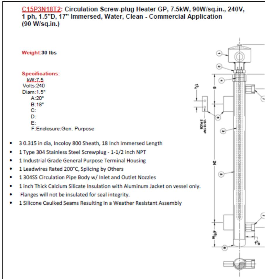
**Figure F-6 Specification of the Heater**
