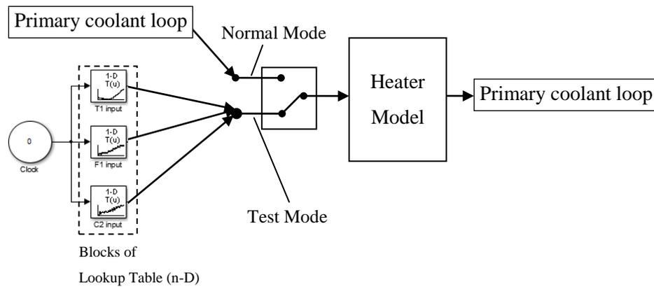
**Figure 5-2 Illustration of the validation method of the Heater**
