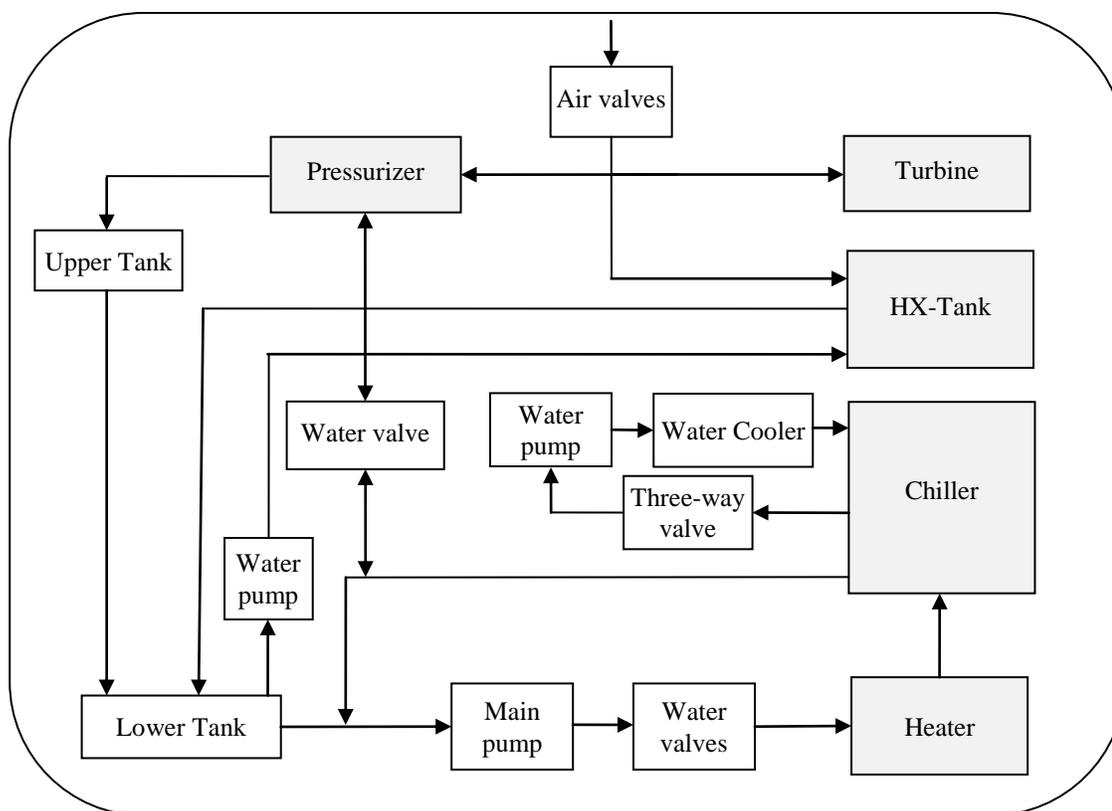
**Figure 1-1 Conceptual scheme of thermal-hydraulic systems of NPCTF**
