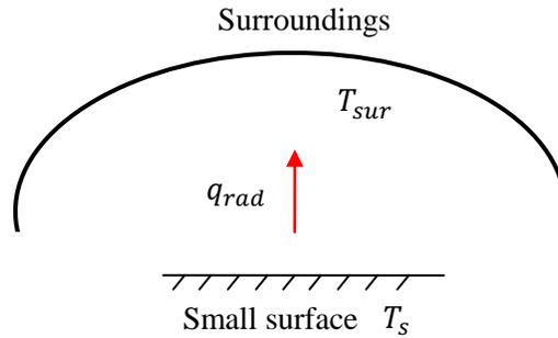
**Figure 2-6: Radiation heat transfer**
