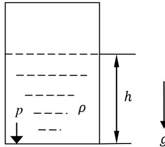
**Figure 2-3 Pressure of a fluid column**
