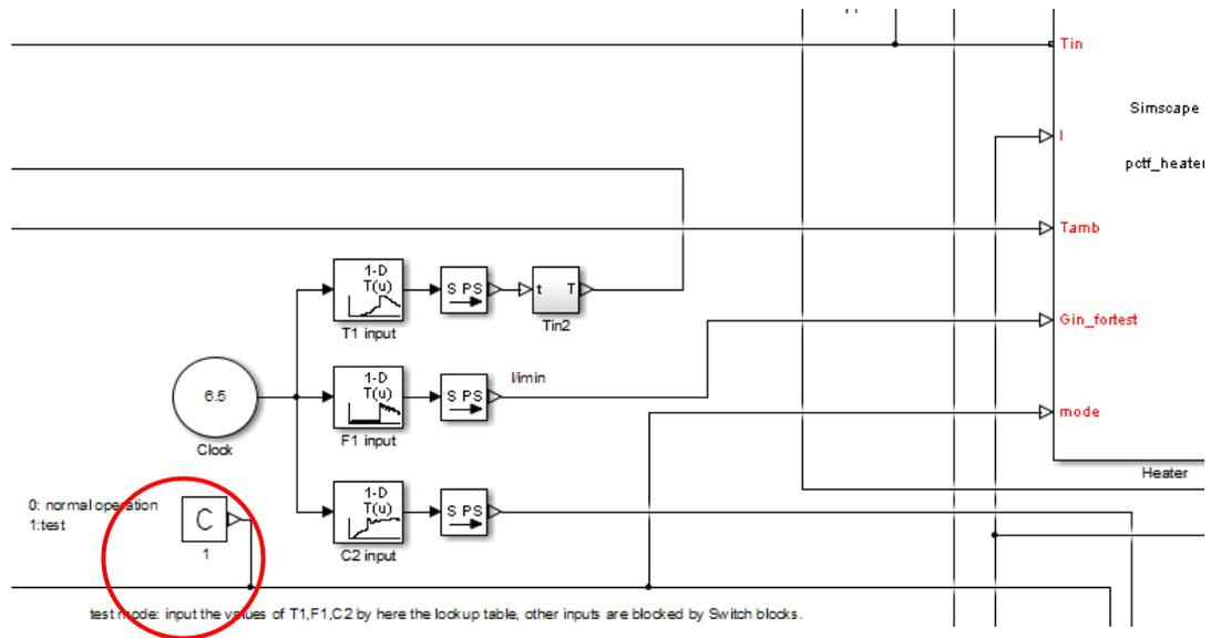
**Figure F-33 Simulation mode of the Heater**
