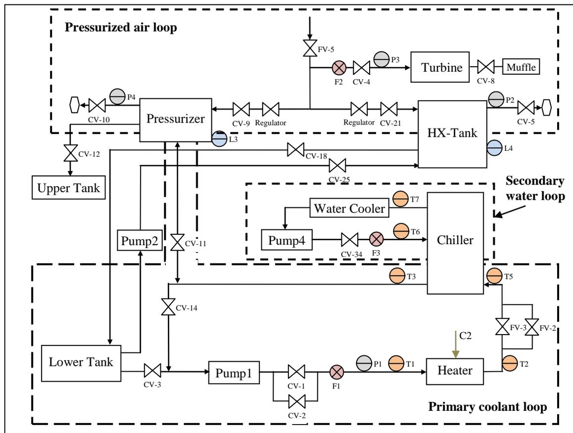
**Figure 2-1 Framework of the simulator**
