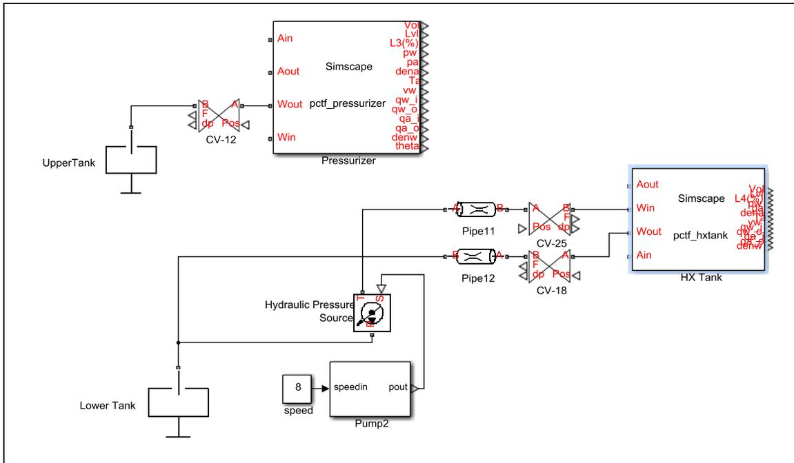
**Figure 4-6 Diagram of the loops for filling and draining water**
