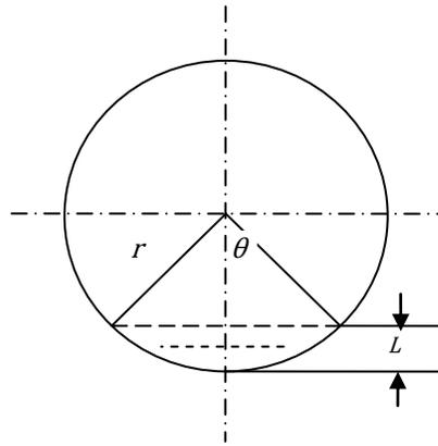
**Figure F-8 Water level of the Pressurizer**
