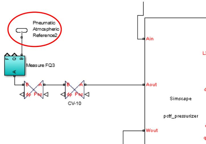
**Figure F-50 Diagram of the air outlet of the Pressurizer**
