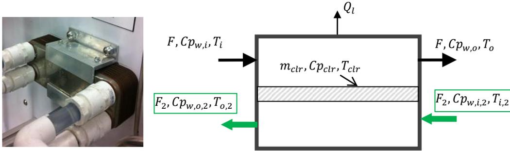
**Figure 2-8 Illustration of the Chiller model**
