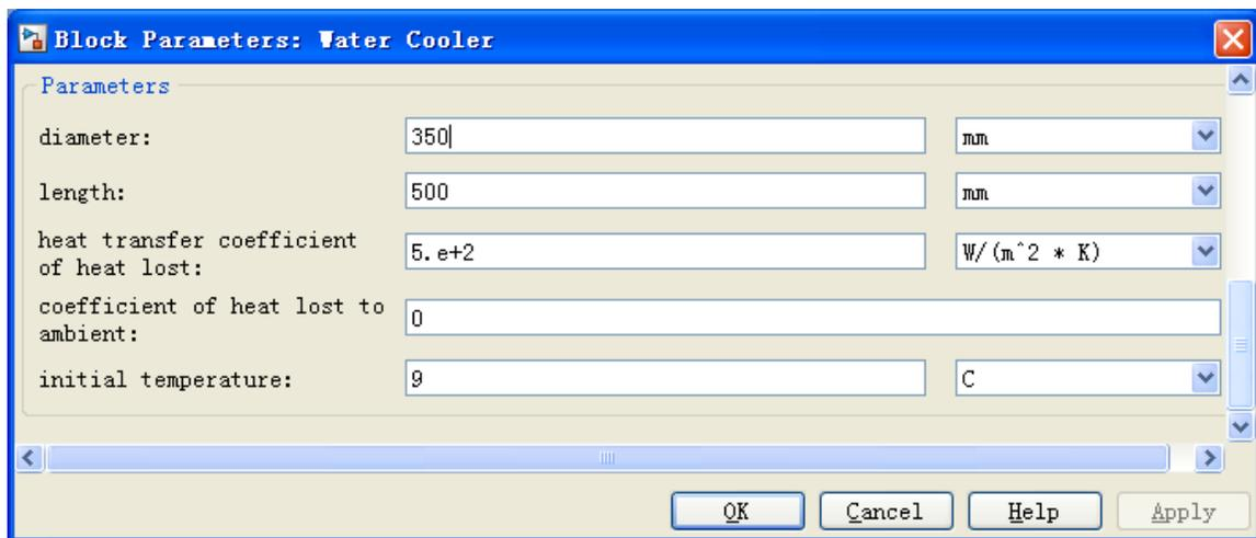
**Figure F-38 Parameter of the Water Cooler**
