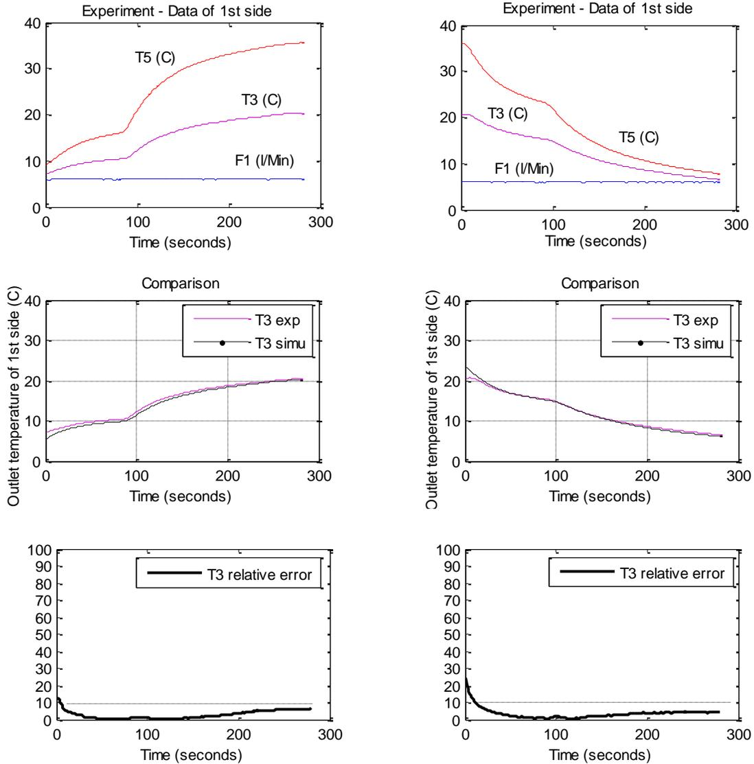
**Figure 5-7 Response of the inlet temperature varying to outlet temperature in the Chiller**
