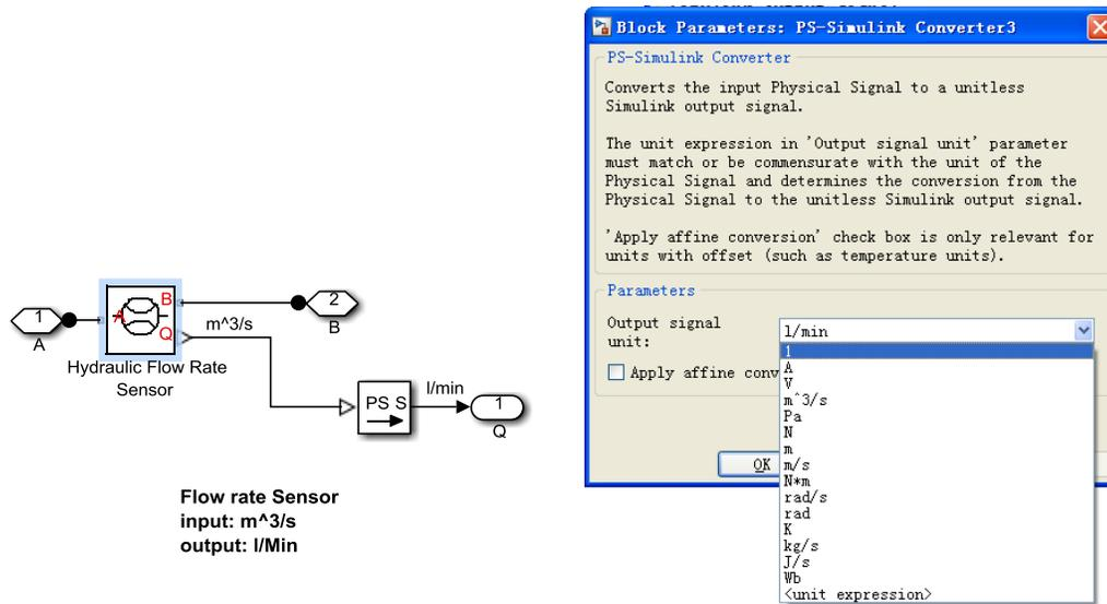
**Figure F-22 Output of hydraulic flow rate sensor**
