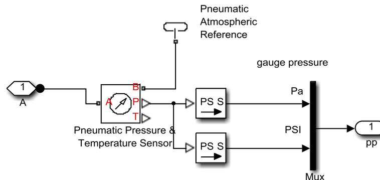
**Figure F-46 Output of pneumatic pressure sensor**
