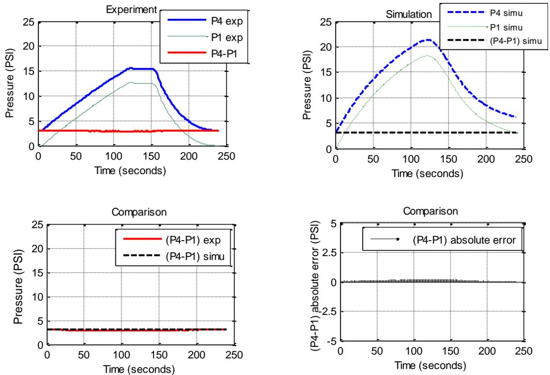
P1 (PSI): water pressure of the primary coolant loop      P4 (PSI): air pressure of the Pressurizer
