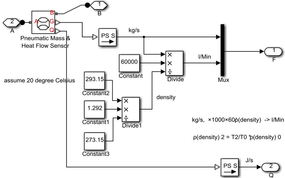
**Figure F-44 Output of pneumatic mass sensor**
