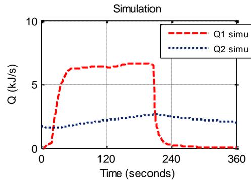
Q1 (kJ/s): heat carried out of the Heater    Q2 (kJ/s): heat released on the secondary side of the Chiller
