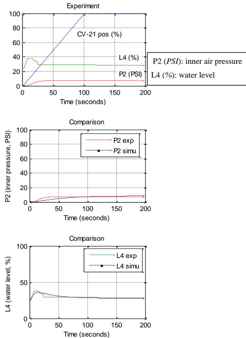
**Figure 5-11 Opening the inlet valve in the HX-Tank**
