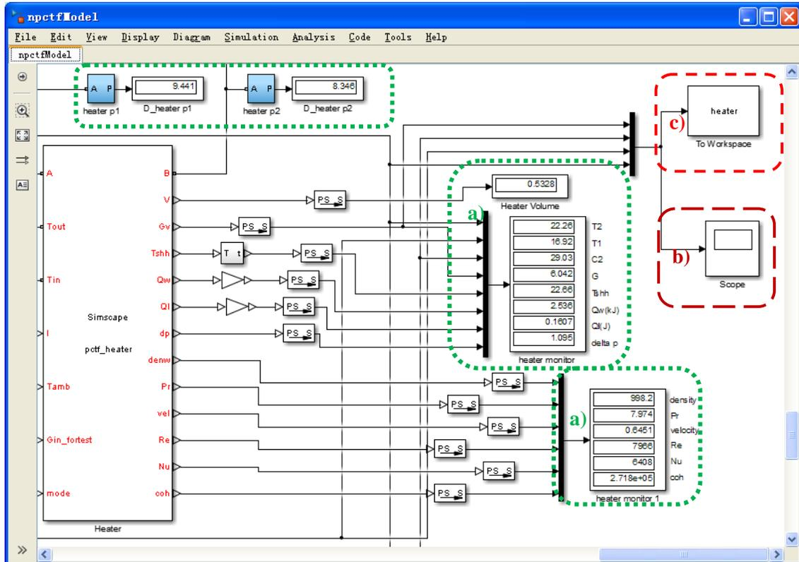
**Figure 4-7 Monitoring simulation variables in the Heater**
