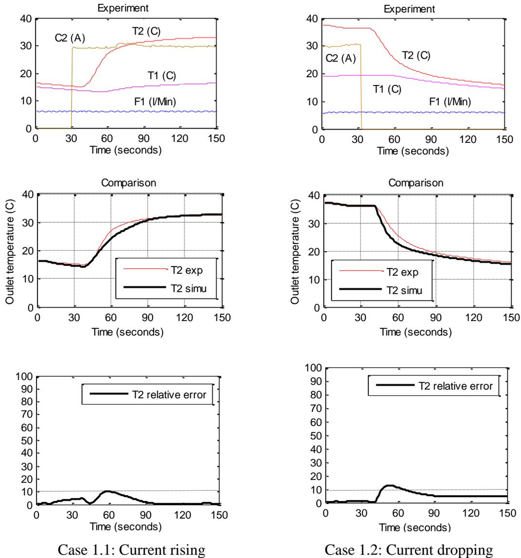
C2 (A): current F1 (l/Min): water flow rate T1 ( °C): inlet temperature T2 ( °C): outlet temperature
