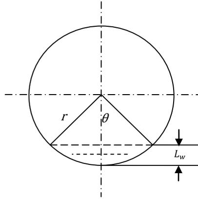
**Figure 2-10 Illustration of the cross of the Pressurizer cylinder**
