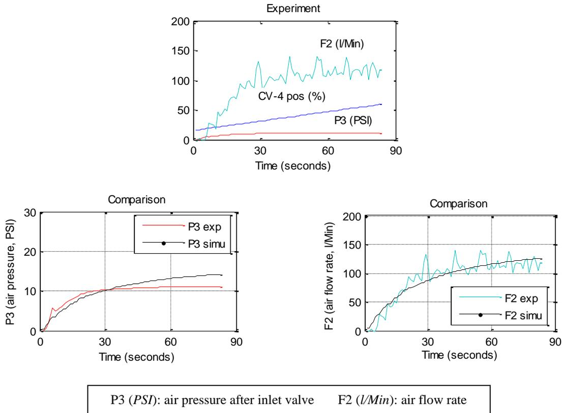
**Figure 5-14 Opening the air inlet valve in the Turbine**
