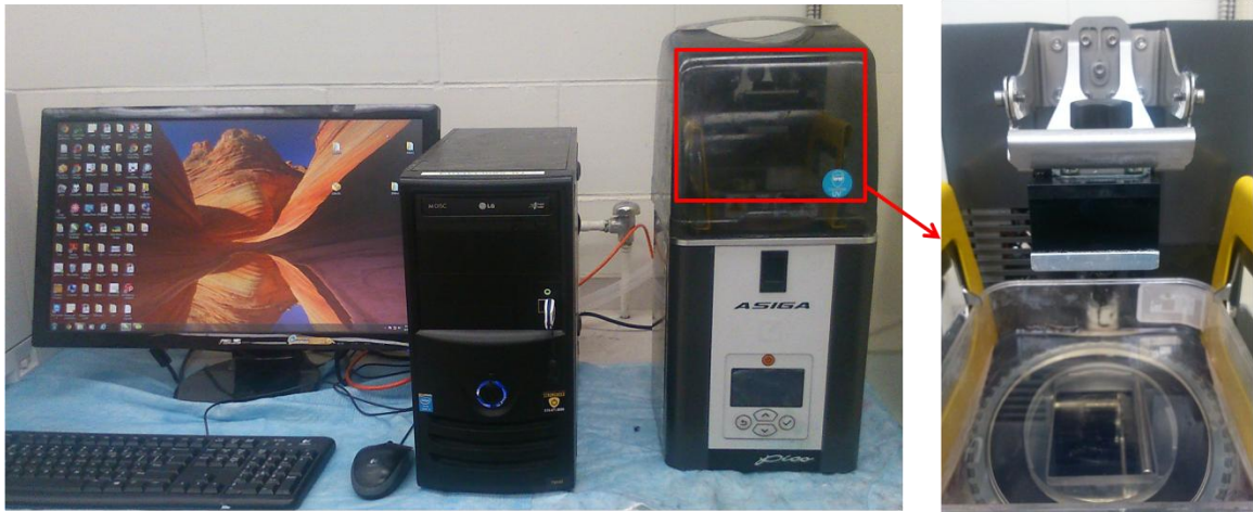
Figure 3.1: Asiga Pico SLA 3D printer and the platform where the 3D structures could be printed.
