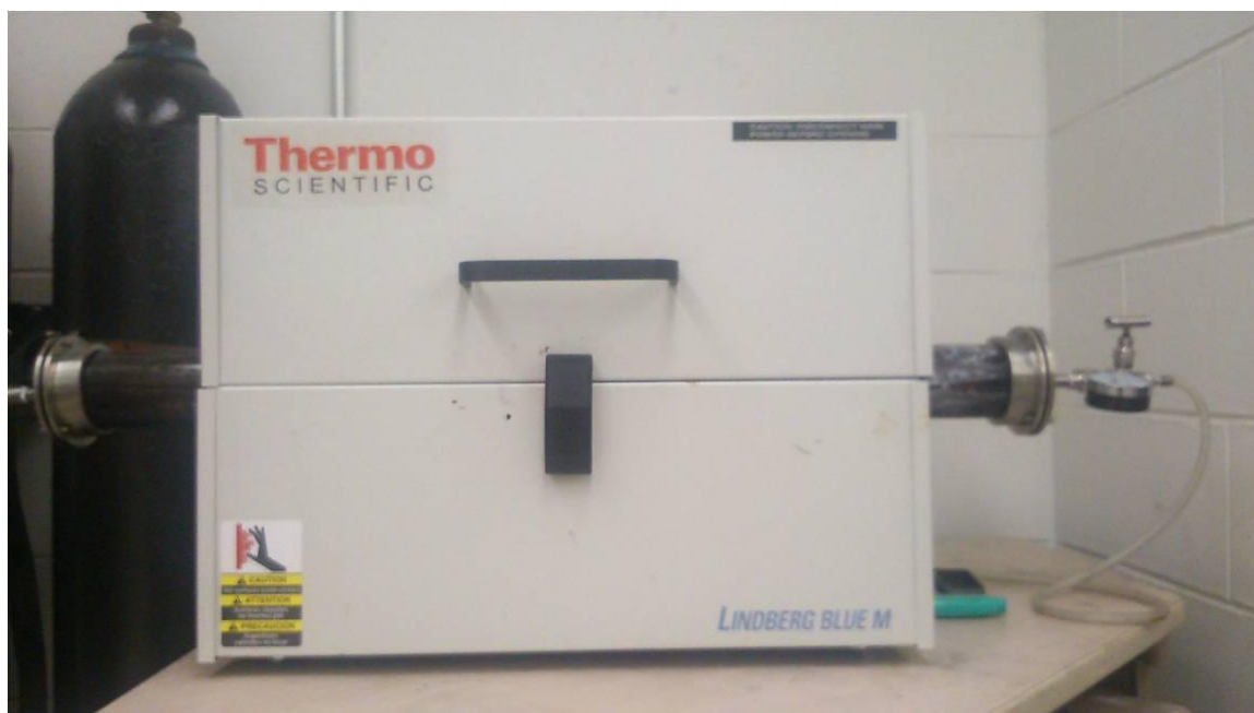
Figure 4.2: Lindberg/Blue M Furnace purchased from Thermo Scientific. Pure nitrogen gas was pumped in during carbonization
