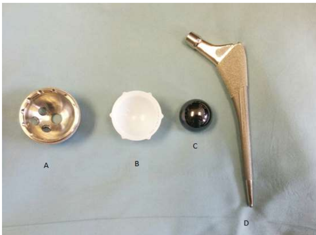
Figure 1-1: Components of a metal-on-polyethylene total hip arthroplasty. A) Acetabular component B) Polyethylene liner C) Femoral Head D) Femoral stem.
