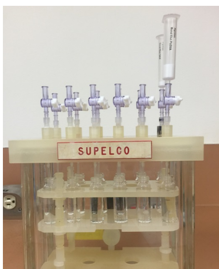
Figure 2.5 SPE procedures using a Bond Elut Plexa cartridge and a Bond Elut SAX cartridge. All of the SPE flow-through solutions were collected into separate scintillation vials. The solutions were to be concentrated for LC-MS 2 analysis.
