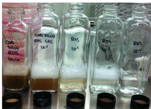
Figure 2.2 Soil dilution bottles (one stock bottle and four dilution bottles) for soil sample plating.
