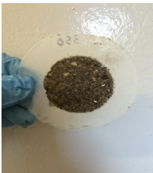
Fig. 4.8: Formation of cake on a filter mesh with TSS of 265 mg/l.
