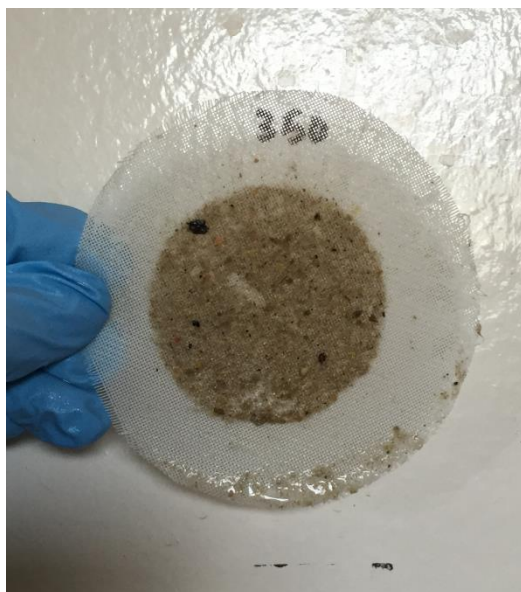
Fig. 4.7: Formation of cake on a filter mesh with TSS of 140 mg/l.
