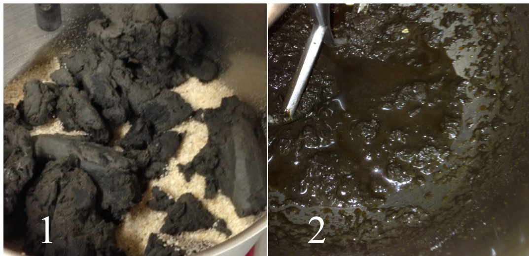
Figure C1: Visual comparison between (1) virgin biosolids resting on top of clean sand and (2) re-wetted biosolids.
