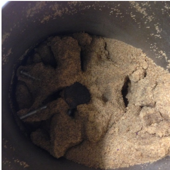
Figure E4: Example photo of the low air permeability crust formed during preheating in Experiment No. 19, which had a very low sand-to biosolids mass ratio but did not blow out.
