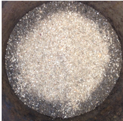
Figure F3: Top down photo of the pyrolysis char edge formed in Experiment No. 8, a self-sustaining experiment.
