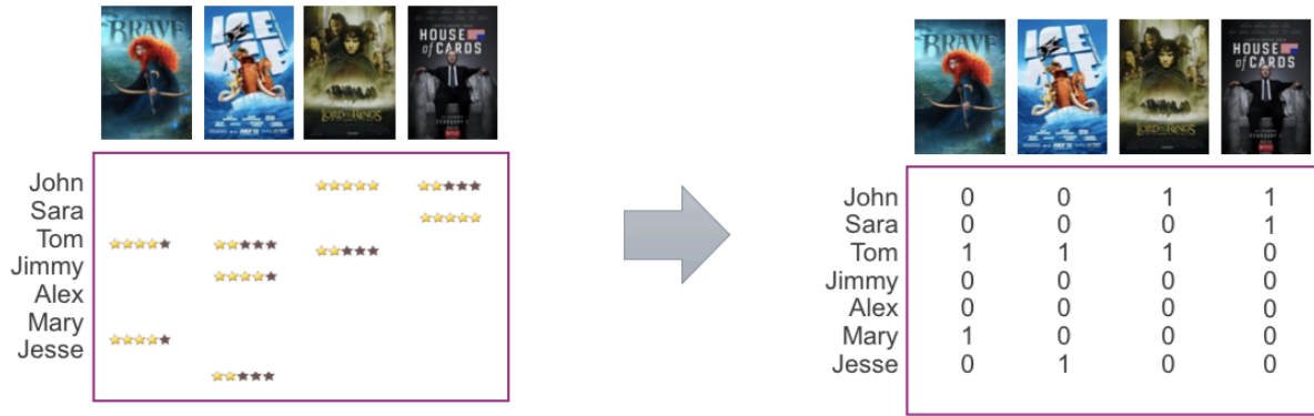
Figure 2.2: Users watch movies that they think they may like. Hence, a rated movie can be considered as an interesting movie for a user.
