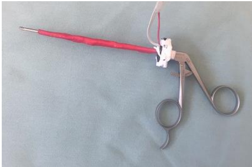
Figure 4.3: The sensorized arthroscopy grasper tool.
