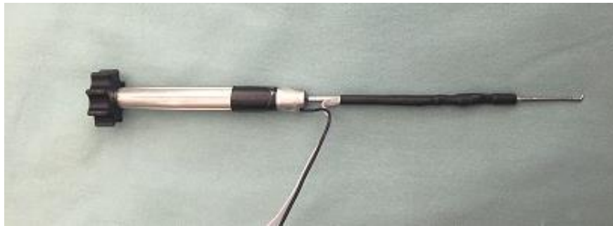
Figure 4.2: The sensorized arthroscopy probe tool.
