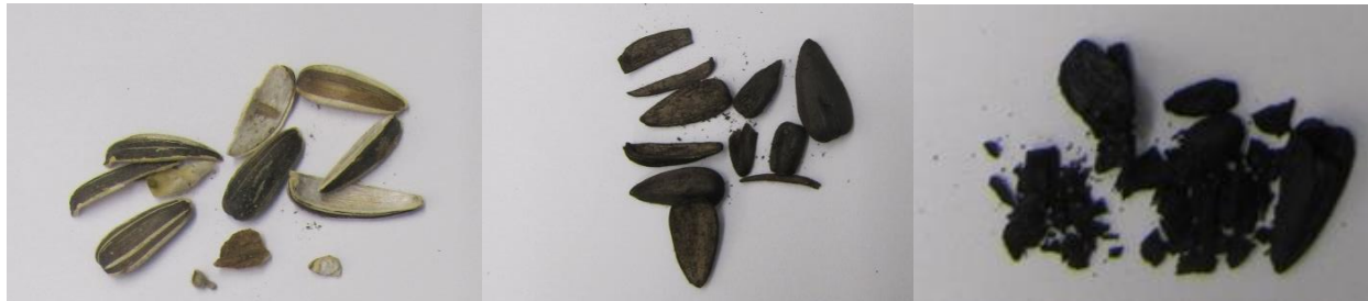
Figure I.10- Example of particle size reduction in the MFR as the torrefaction temperature is increased to 300 °C
