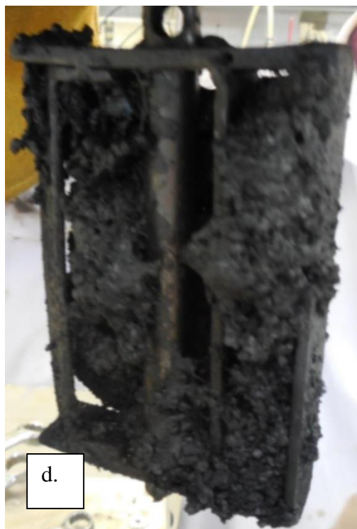
Figure I.4- Morphology of sorghum particles a. untreated b. torrefied at 260 °C c. popping of the seeds at 300 °C, d. stirrer after torrefaction at 300 °C
