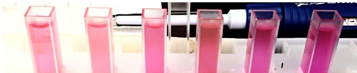
Figure 2.13- Colorimetric reaction of Rhodamine 6G with tetraiodomercurate
