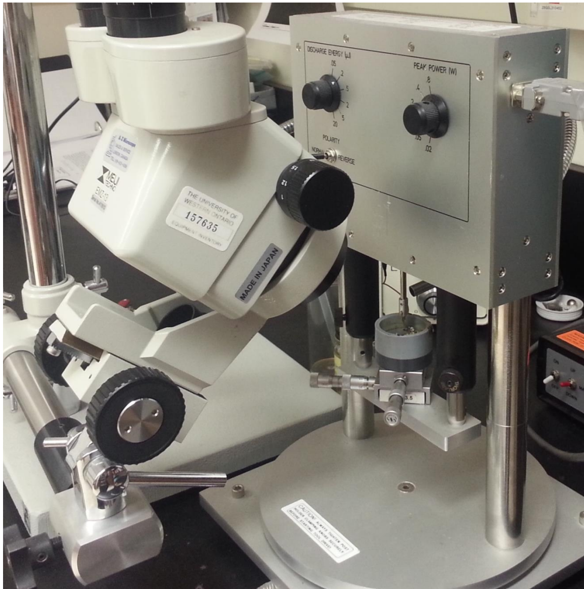
Figure 2.10: Electronic drilling machine (EDM).
