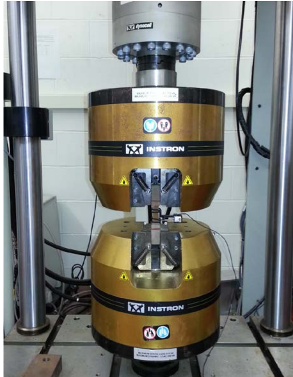
Figure 2.25: Cyclic test set-up of RPF sample
