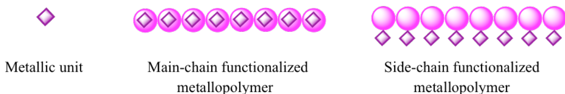
Figure 1.12. Schematic representation of a main-chain and a side-chain functionalized metallopolymer.
