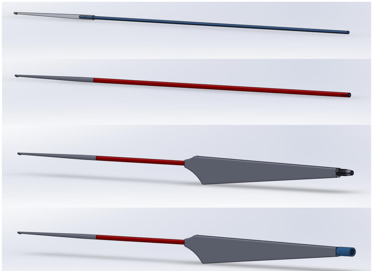
Figure 3.16: CAD probe assembly view (top to bottom) slotted sensor shaft (blue) with tapered tip attachment; outer shaft (red); triangular handle with colleted end; securing bolt (blue)
