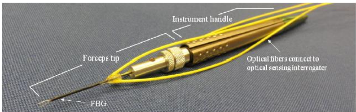
Figure 2.7: 2-DOF force sensing micro-forceps [27].
