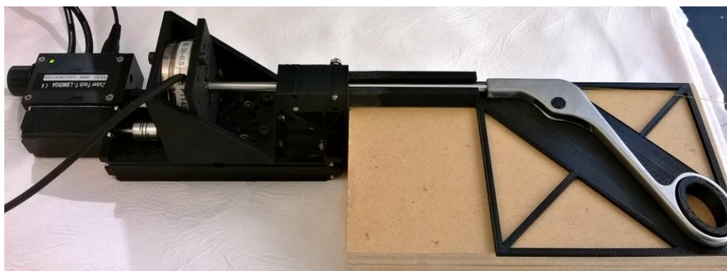
Figure 4.1: Axial calibration apparatus.
