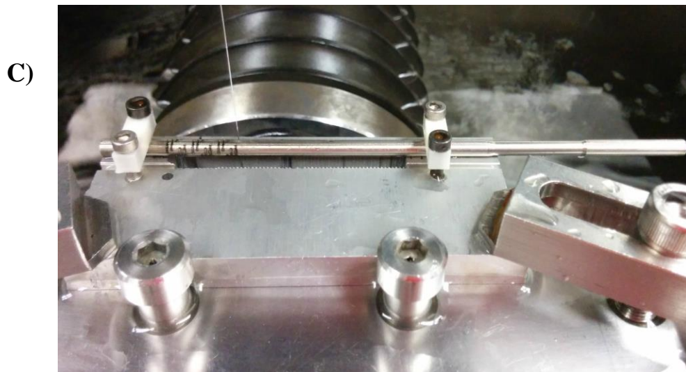
Figure 3.8: Axial amplification element (a) SolidWorks model; (b) EDM manufactured model; (c) EDM setup.
