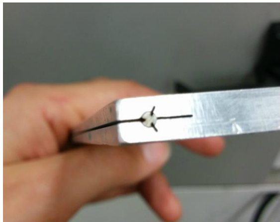
Figure 3.20: Probe clamp (a) EDM setup; (b) final grooves.
