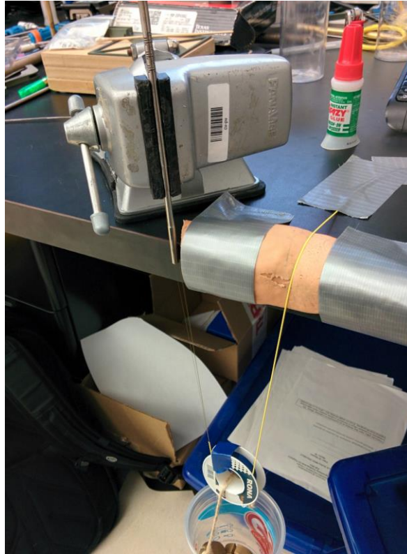
Figure 5.3: FBG pre-straining apparatus.
