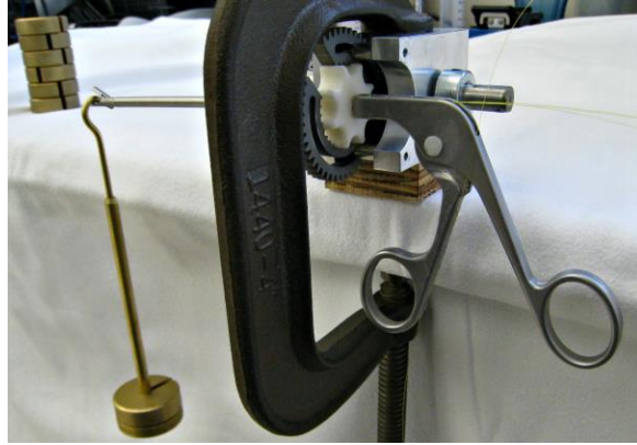
Figure 4.2: Bending calibration apparatus.
