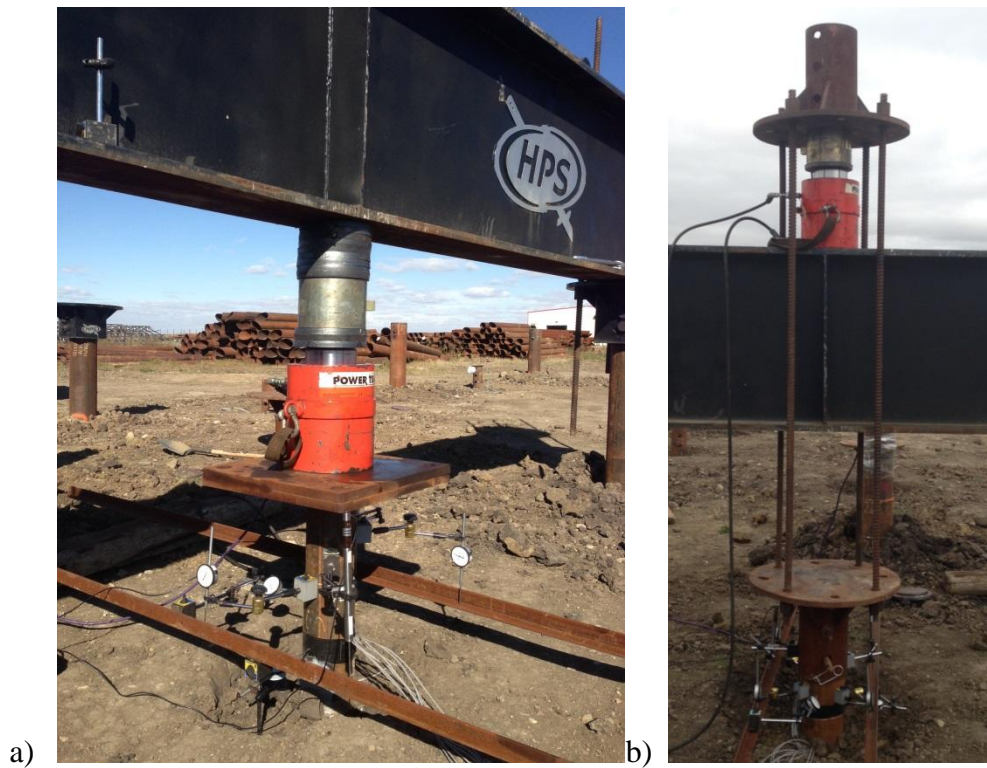
Figure 5-1: Loading Setup a) Compression b) Tension
