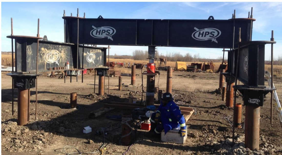
Figure 5-2: Reaction Setup a) Two Reaction Pile Setup b) Four Reaction Pile Setup
