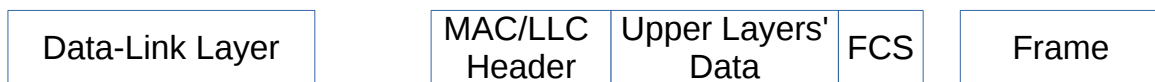
Figure 2.10: Data-Link Layer Frame Formulation by Header and Trailer Encapsulation of Upper Layers' Data
