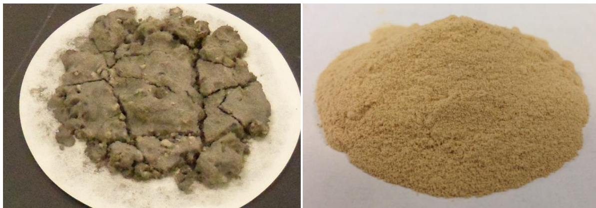
Figure 6.4 Photographs of solid residue from HL depolymerization at 200 °C with MoRu/AC catalyst (left) and HL feed before reaction (right)
