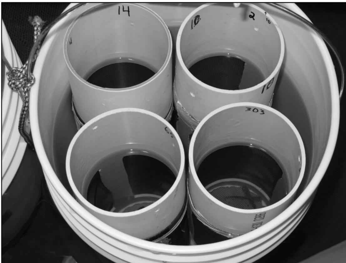
**Figure 9.** Photo of apparatus for the 24-hour saltwater challenge. Each Bucket was immersed in 11 °C aerated water (24 ppt). Each of four cups had five fish from each container in the tanks.
