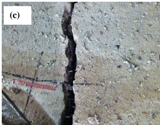
(c) Steel fibres rupture failure mechanism
