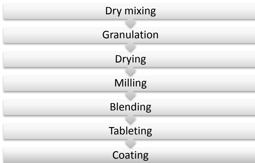
Figure 3.2: Schematic of pharmaceutical tablet manufacturing pathway (Adapted by Summers et al. [4])
