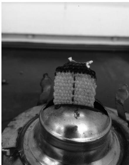
**Figure 3.13: Wick consumption with inadequate fuel. Pyrolysis sample obtained at 450 C**
