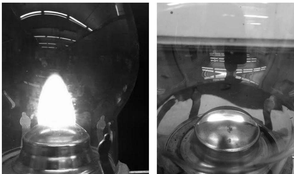
**Figure 3.14: Insufficient fuel supply in a traditional wick lamp. (left) initial ignition, (right) flame diminishing. Pyrolysis sample obtained at 450 C**
