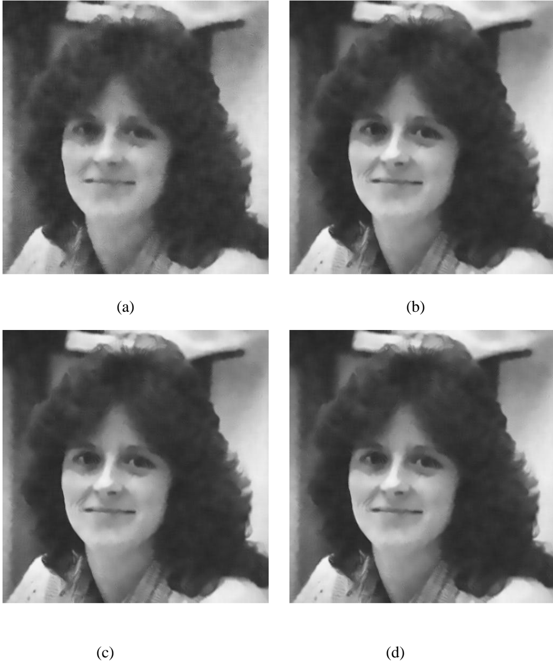
Figure 3 - 3: Performance analysis using Woman 1 image over different search region sizes where noise level is \sigma=40 (a) search region size= 14\times 14 , PSNR = 29.11, (b) search region size= 21\times 21 , PSNR = 29.78, (c) search region size= 28\times 28 , PSNR = 29.78, and (d) search region size= 35\times 35 , PSNR = 29.79.
