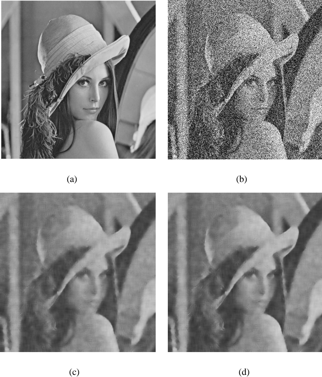
Figure 4- 10: Subjective comparison for denoising performance for Non-Local Means at noise level \sigma=100 . (a) Noise free image Lena, (b) noisy image with Additive white Gaussian noise, (c) denoised image using the NLM method , PSNR= 22.18, and (d) denoised image using the proposed method, PSNR = 22.29.
