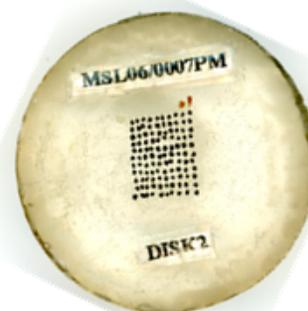
**Figure 1-5: Selected polished probe chromite mount approximately 2.5 cm across**
