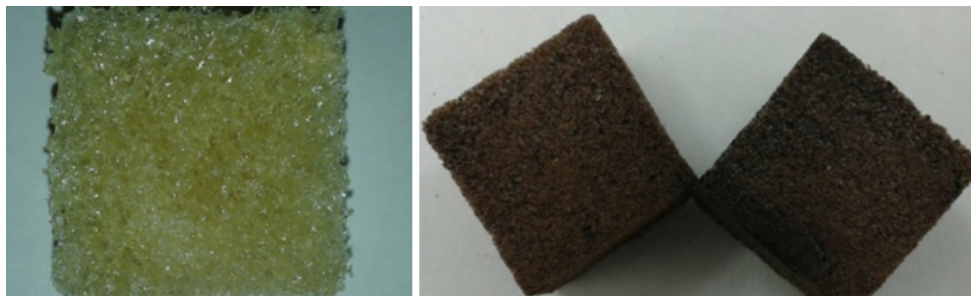
Figure 7-3 PU foams with 100% PPG400 and glycerol (left) and bio-PU foams with 50% replacement of PPG400 with DHL (right)
