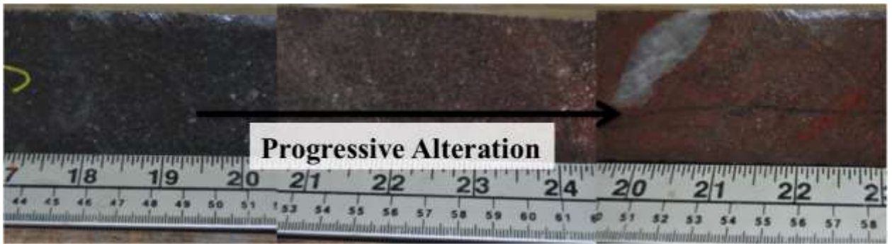
Figure 4.11: Progressive alteration of the Thunder Creek stock. Moving from unaltered (left) to strongly altered (right).
