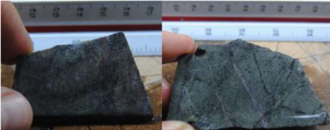
Figure 5.1: Hand sample photographs of alteration in Thunder Creek mafic volcanics. On the left is an altered volcanic sample. The right is a least altered sample. The sample on the left has visible iron carbonate staining (brown).
