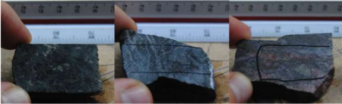
Figure 5.4: Hand sample images of the Thunder Creek pyroxenite becoming increasingly altered moving right.
