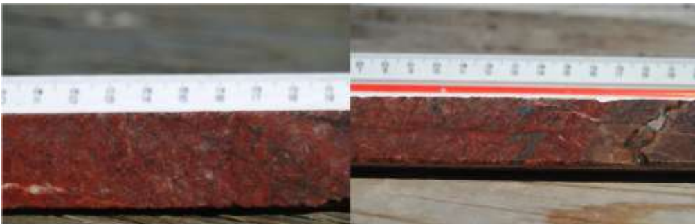
Figure 5.17: Two hand sample photographs of the dark red altered syenite. The photo on the right side contains a carbonate altered bleached zone in the right corner.
