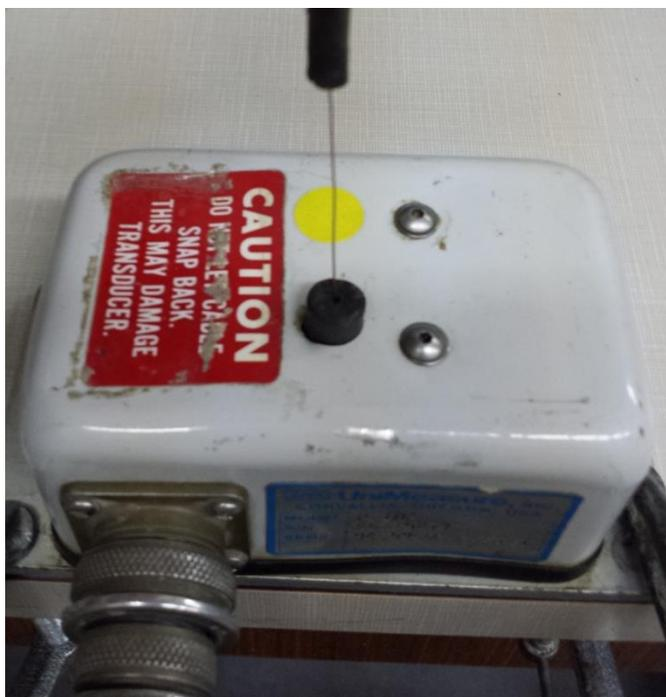
Figure 3.30. Typical string pot used to measure the consolidation settlement for the clay.
