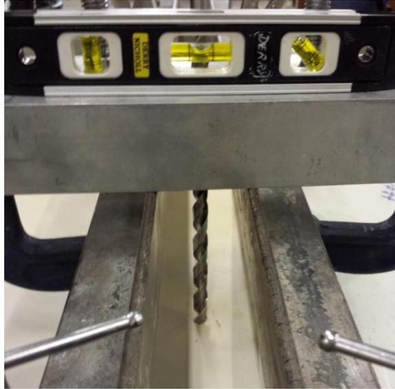
Figure 3.42. Process used to install the micropile in clay.
