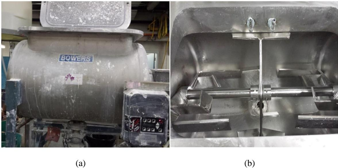
Figure 3.15. Clay slurry mixer; (a) outside view and (b) inside.
