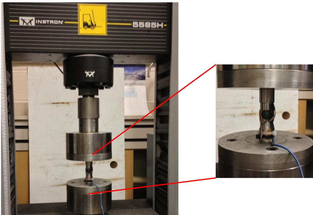
Figure 3.23. Calibration process for the primary load cell using the compression machine.
