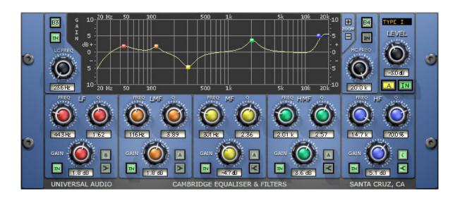
Figure 2.1 UAD's Cambridge EQ can be used to notch out offensive frequencies
