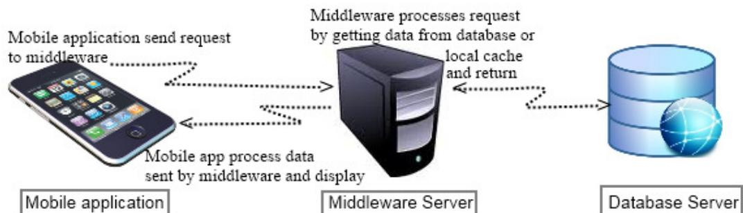
**Figure 4-1: High level overview of the system**
