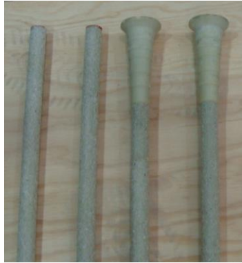
Fig. 1 View of HM-GFRP bar with end anchorage head
