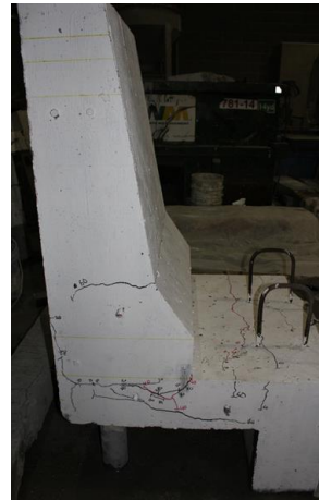
a) Crack pattern at the right side of the specimen b) Crack pattern at the left side of the specimen Fig. 10. Views of crack pattern for specimen S-1 after failure
