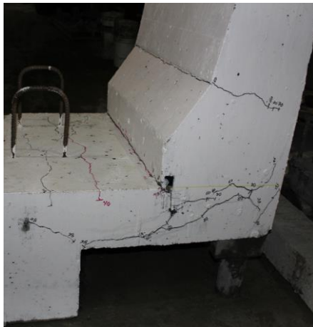
a) Crack pattern at the right side of the specimen b) Crack pattern at the left side of the specimen Fig. 10. Views of crack pattern for specimen S-1 after failure
