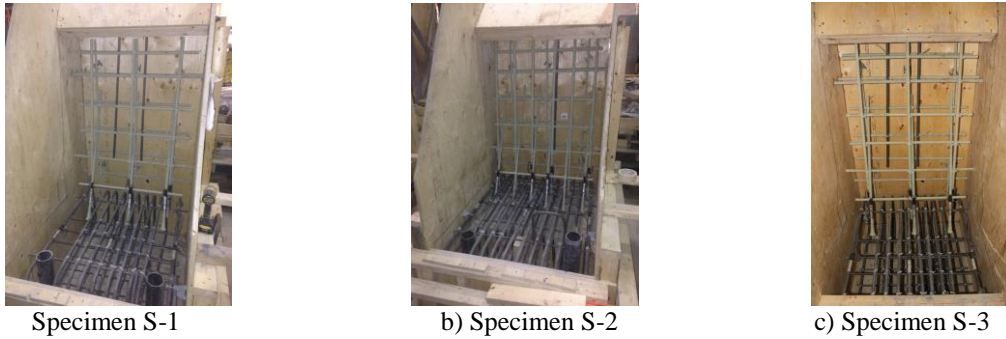
Fig. 7. View of internal reinforcement in the tested barrier specimens
