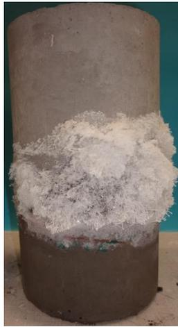
Figure 1: Salt crystals on concrete surface
