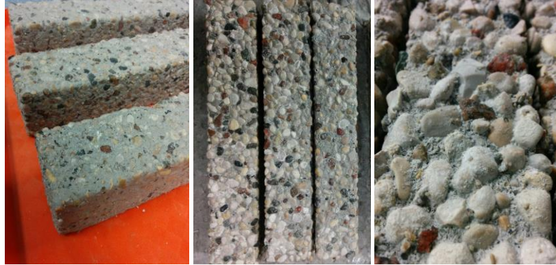
Figure 1: Features of damage of concrete specimens immersed in the 5% sulfuric acid solutions after 1 (left), 7 (middle) and 13 (right) weeks.
